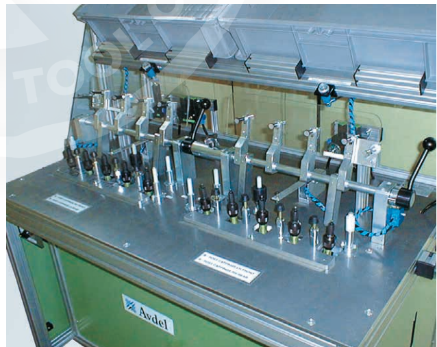
10 placing heads to assemble automotive sealing strips
