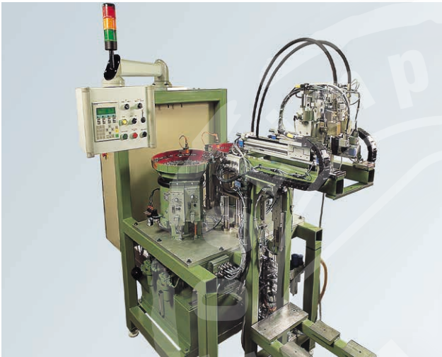
MIRS System to assemble vacuum pump
